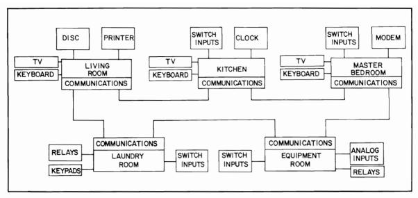
Fig. 8-1. Five areas of a computer-controlled house. Separate microprocessor-based nodes communicate via an intelligent communications processor and an advanced data link controller.
